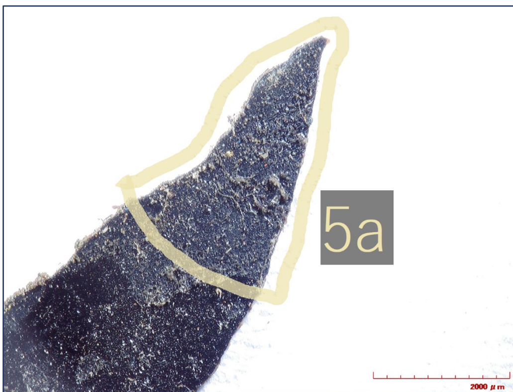
Figure 12-13: Hirox KH-7700 3-D Digital Microscope Image of Sample Taken from Sampling Site Five (x40), Part 5a outlined here selected for embedding
